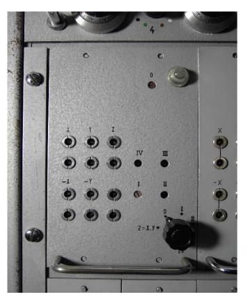
The following picture shows the right hand side of such a multiplier (showing the output amplifier):
