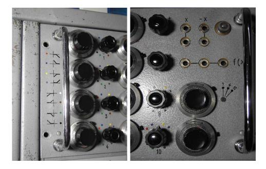
The multipliers of the prototype are of the parabola type, i.e. they rely on the fact that  $4xy = (x + y)^2 - (x - y)^2$ . The square functions are generated by using diode based polygon function generators as shown below (see [8][p. 143]):
