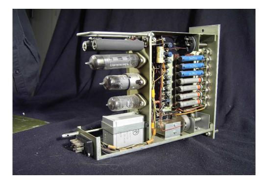
Telefunken used a high speed relay to reset this amplifier circuit:
